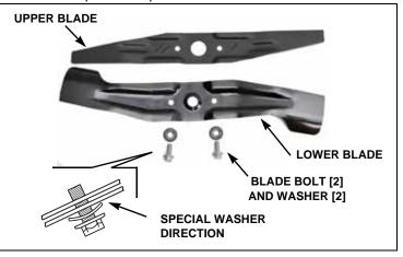
4. Tighten the blade bolts with a torque wrench to the specified torque. Use a wooden block to prevent the blades from turning when tightening the bolts, as shown on page 12.
