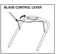
Release the blade control lever to stop the engine and stop blade rotation whenever you need to leave the mower.
