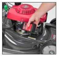
If you don't use the supplied oil, add enough SAE 10W-30 API service category SJ or later oil to bring the oil level between the upper and lower limit marks on the dipstick—without screwing the dipstick in (approximately 12 to 13.5 ounces is required) See page 6.
