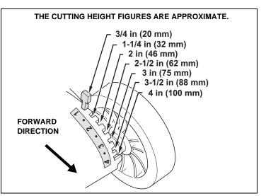
If you are not sure what cutting height to select, start with a high setting and check the appearance of the lawn after mowing a small area. Then readjust the cutting height if necessary.
