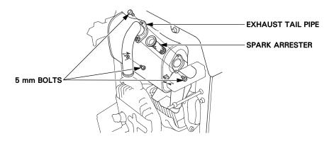
7. Use a brush to remove carbon deposits from the spark arrester screen.
