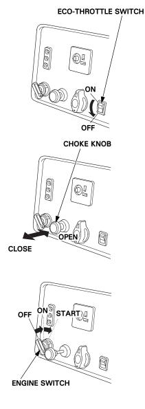
6. If the choke knob was moved to the CLOSED position to start the engine, gradually push it to the OPEN position as the engine warms up.
