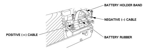
4. Remove the battery and the battery rubber from the battery tray.
