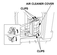
3. Check the foam air filter and paper air filter to be sure they are clean and in good condition. If the foam air filter is dirty, clean it as described on page 48. Replace the foam air filter if it is damaged.
