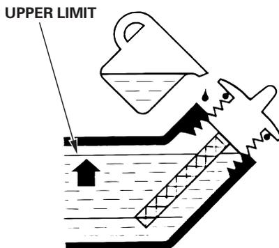
The Oil Alert system will automatically stop the engine before the oil level falls below safe limits. However, to avoid the inconvenience of an unexpected shutdown, check the oil level regularly.
