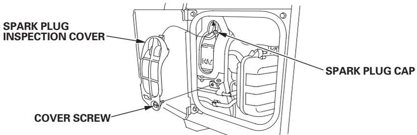
3. Remove the spark plug cap.
