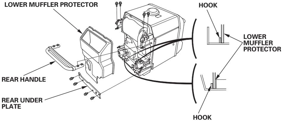
Install the lower muffler protector inside the hook securely.
