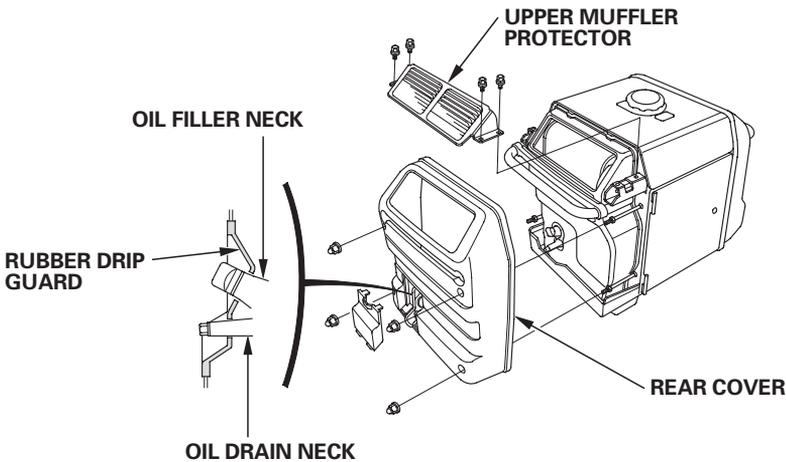
When installing the rear cover, carefully fit the rubber drip guard around the oil filler neck and oil drain neck.
