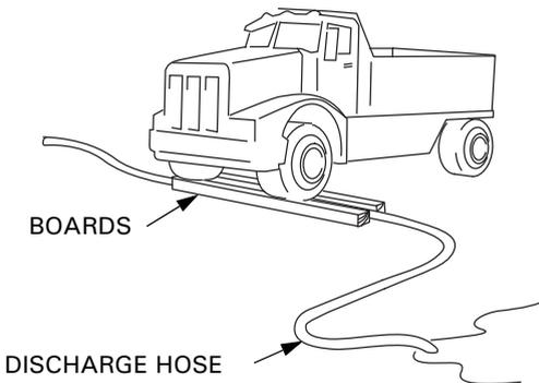
Driving over a discharge hose while the pump is running, or even possibly when the pump is stopped, may cause pump case failure.
