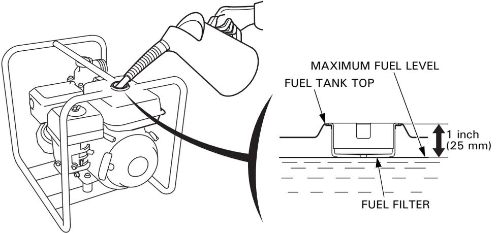
Refuel in a well-ventilated area before starting the engine. If the engine has been running, allow it to cool. Refuel carefully to avoid spilling fuel. Do not fill the fuel tank completely. Fill tank to approximately 1 inch (25 mm) below the top of the fuel tank to allow for fuel expansion. It may be necessary to lower the fuel level depending on operating conditions.
