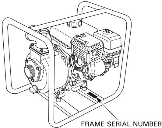
Record the frame serial number (if assigned) and the engine serial number in the space below. You will need these serial numbers when ordering parts, and when making technical or warranty inquiries (see page 59).
