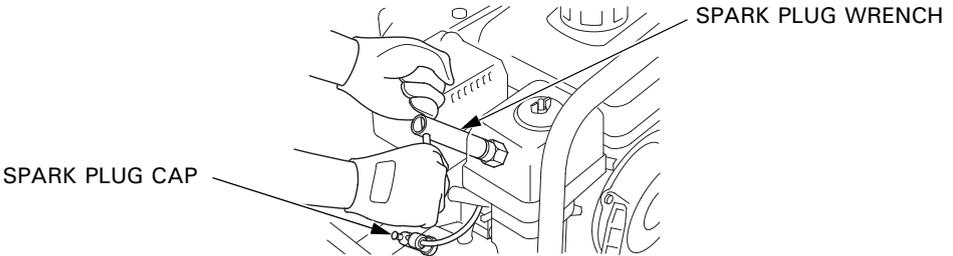
3. Inspect the spark plug. Replace it if the electrodes are worn, or if the insulator is cracked or chipped.
