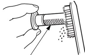
5. Install the spark arrester, muffler protector, and muffler in the reverse order of disassembly using a new gasket.
