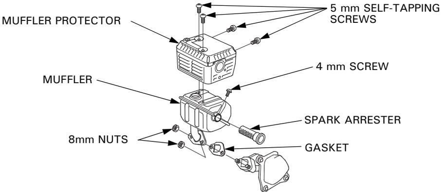
4. Use a brush to remove carbon deposits from the spark arrester screen. Be careful to avoid damaging the screen.
