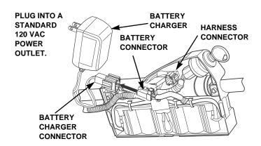
4. Plug the charger into a standard 120 Vac power outlet and let the battery charge for 20 to 24 hours. The charger may become slightly warm during charging. This is normal.
