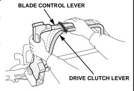
move gradually faster as you push the drive clutch lever forward. If you push the lever all the way forward to the handlebar, the mower will move at the speed determined by the shift lever setting (below).
