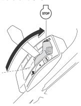
HZA model: turn the key switch to the OFF position.
