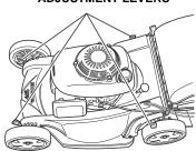
To adjust cutting height, pull each adjustment lever toward the wheel, and move it into another notch.
