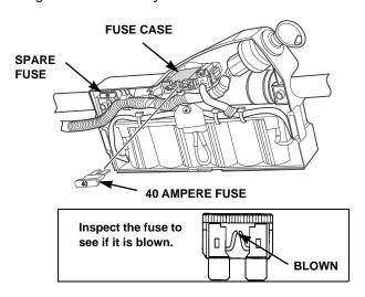
If a frequent fuse failure occurs, it usually indicates a short circuit or an overload in the electrical system. Take the mower to an authorized Honda servicing dealer for repair.
