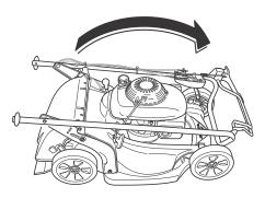
When unfolding the handlebar, be sure to lock the adjust knobs to secure the handlebar in the mowing position (see <u>page 3</u>).
