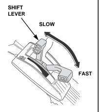
For maximum mowing performance, use the lower speed range for mowing and the higher speed range for transporting.
