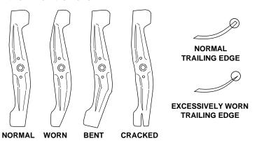
If a blade is bent, take the lawn mower to an authorized Honda servicing dealer for inspection.
