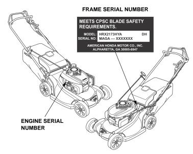
There are two serial numbers, one for the engine and one for the mower frame. Record the engine and frame serial numbers in the space below. You will need these serial numbers when ordering parts and when making technical or warranty inquiries (page 20).
