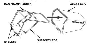
Install the plastic clips over the bag frame as shown.
