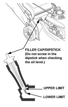
Do not overfill the engine with oil. If the engine is overfilled, the excess oil may get transferred to the air cleaner housing and air filter.
