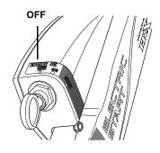
When the mower is not in use, turn the fuel valve to the OFF position.
