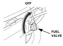
4. If your equipment will not be used for 3 to 4 weeks, we recommend running the engine's carburetor out of fuel. You can do this by leaving the fuel valve OFF, restarting the engine and running it out of fuel. See "Fuel" on page 16 for periods of inactivity that exceed 4 weeks.
