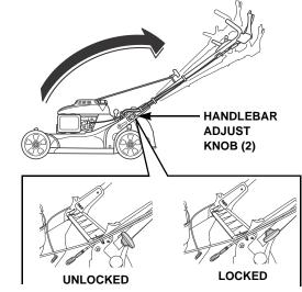
Turn the adjusting knobs 90 degrees into the lock position and the pins will spring into the holes and lock into position.
