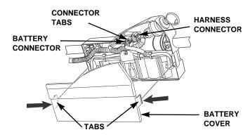
Connect the battery connector to the charger supplied with the mower.
