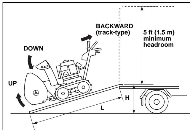
4. After the snow blower is in the truck, stop the engine, and turn the fuel valve to the OFF position. This will prevent the possibility of carburetor flooding and will reduce the possibility of fuel leakage.
