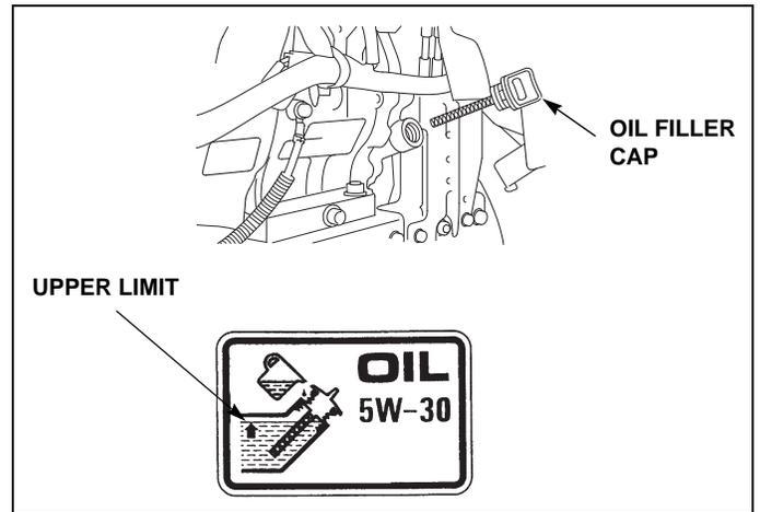
1. With the snow blower on a level surface, remove the oil filler cap/dipstick.
