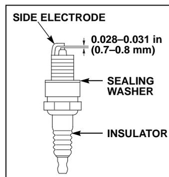
7. After the spark plug is seated, tighten with a spark plug wrench to compress the washer.
