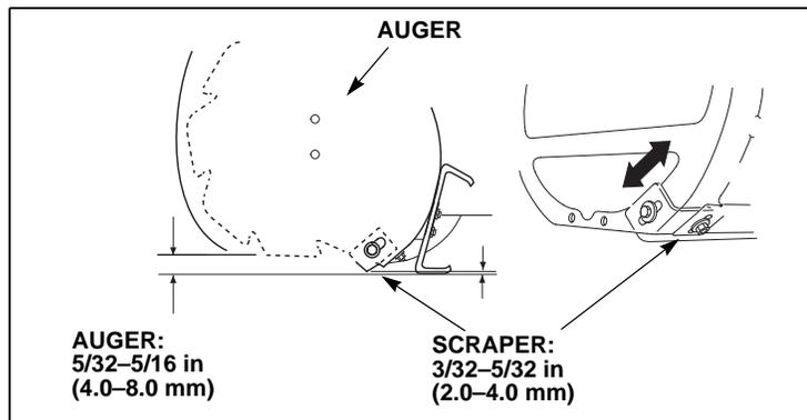
Adjust the scraper equally on both sides so that it remains parallel with the ground. Be sure to tighten the scraper bar bolts and nuts after making adjustments.
