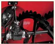
**Heavy-Duty, Serrated Augers** lce-breaking augers automatically lift in reverse when Automatic or Semi-Automatic modes are engaged.
