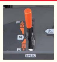
Control of forward and reverse speed is simplicity itself with Honda's hydrostatic transmission — standard on HSS724, HSS928 and HSS1332 series snow blowers. A single lever accurately adjusts ground speed without affecting auger rotation speed. The farther you move the lever, the faster your Honda Snow Blower moves — push forward to move ahead or pull back for reverse.
