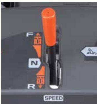
Control of forward and reverse speed is simplicity itself with Honda's hydrostatic transmission — standard on HSS724, HSS928 and HSS1332 series snow blowers. A single lever accurately adjusts ground speed without affecting auger rotation speed. The farther you move the lever, the faster your Honda Snow Blower moves — push forward to move ahead or pull back for reverse.
