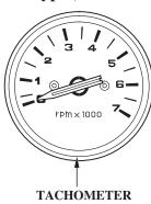
The tachometer shows engine speed in revolutions per minute.
