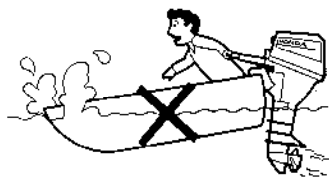
INCORRECT CAUSES BOAT TO "PLOW"
