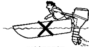
INCORRECT CAUSES BOAT TO "PLOW"
