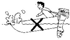
INCORRECT CAUSES BOAT TO "PLOW"
