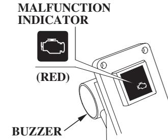
When the engine control system detects an engine control system malfunction, the malfunction indicator turns on and the buzzer sounds at one-second intervals.
