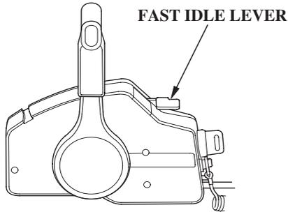
Use the fast idle lever to accelerate engine warm-up after starting the engine. Do not use the fast idle lever when starting the engine.
