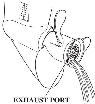
5. Turn on the fresh water supply and flush the outboard motor for at least 10 minutes.
