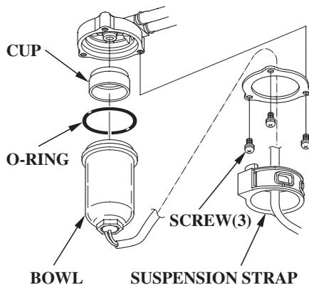
5. Remove the three screws and separate the water separator cup from the body.
