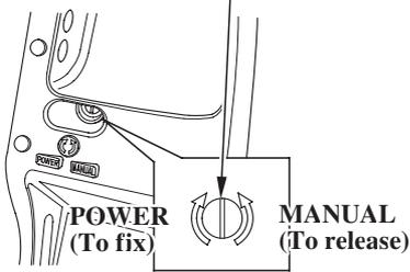
The outboard motor can be tilted manually after opening the manual relief valve. This allows the outboard motor to be tilted up or down when no battery is connected.
