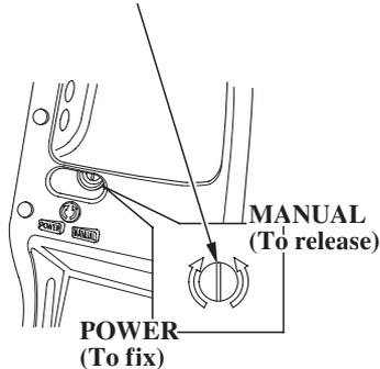
The outboard motor can also be tilted manually after opening the manual relief valve. This feature enables the outboard motor to be tilted up or down when no battery is connected.
