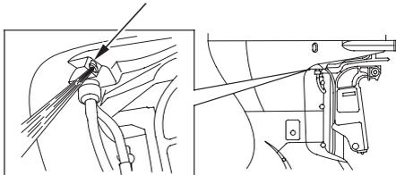
If overheating activates the engine protection system, idle the engine in neutral, and check the cooling system indicator.
