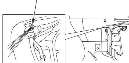
Water should flow from the cooling system indicator while the engine is running. This shows that water is circulating through the cooling system.
