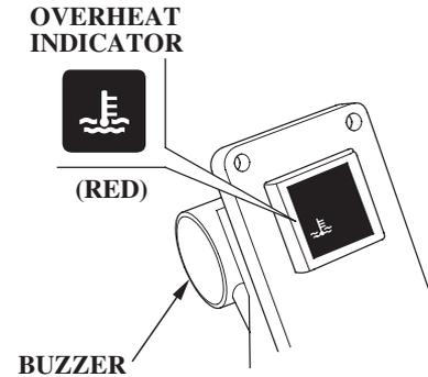
When the alert triggers, the overheat indicator comes on and the buzzer sounds a steady tone as the engine speed is reduced to 1,800 rpm. If the condition persists for another 20 seconds, the engine shuts off. Refer to *TAKING CARE OF UNEXPECTED PROBLEMS*, on p. 99 .
