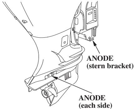
The anodes are located on each side of the gear case. They are made of a sacrificial material that helps to protect the outboard motor from corrosion.
