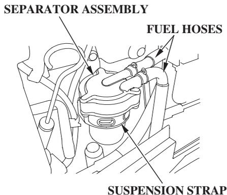
3. Remove the suspension strap from the water separator bracket; then remove the strap from the separator assembly. During removal of the separator assembly, take care not to damage the wire harness with the separator bracket.
