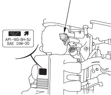
4. If the oil level is low, remove the oil filler cap, and add oil to reach the upper limit mark shown on the dipstick. Use the oil recommended on p. 68.
