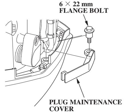
3. Remove the 6 × 22 mm flange bolt and remove the plug maintenance cover.
