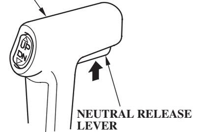
The gearshift/throttle control lever controls engine speed and selects F (forward), N (neutral), or R (reverse) gears.
