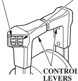
The power trim/tilt switch is located on the control lever. It is a rocker switch with UP and DN (down) positions for changing the angle of the outboard motor.
