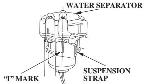
8. Align the “I” mark on the suspension strap as shown above and install the water separator to the bracket.
