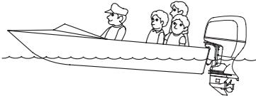
If steering effort is not equal in both directions, adjust the trim tab to compensate for “torque steer,” which is the reaction of the outboard motor to propeller rotation.
