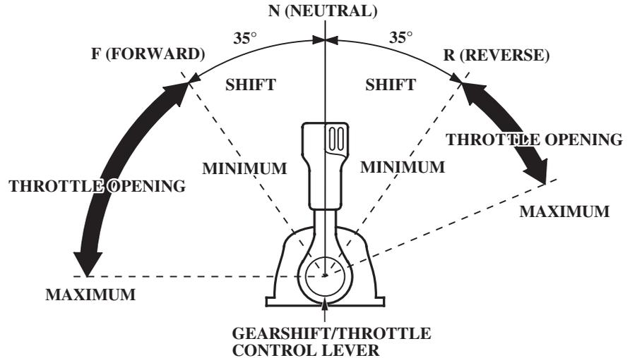
Moving the control lever 35° from N (neutral) selects the gear, and further movement increases engine speed.
