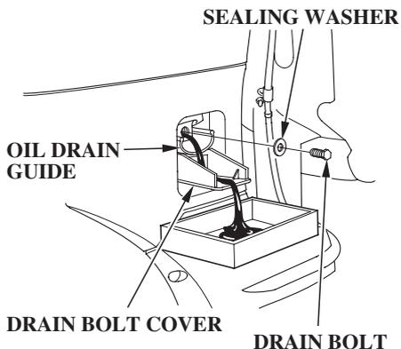
3. Set the drain bolt cover under the guide.
