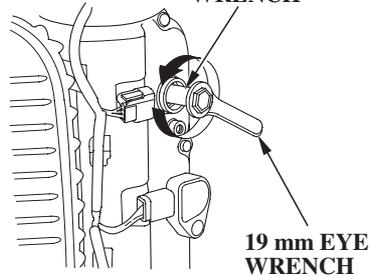
6. Remove the spark plugs with a spark plug wrench and 19 mm eye wrench.
