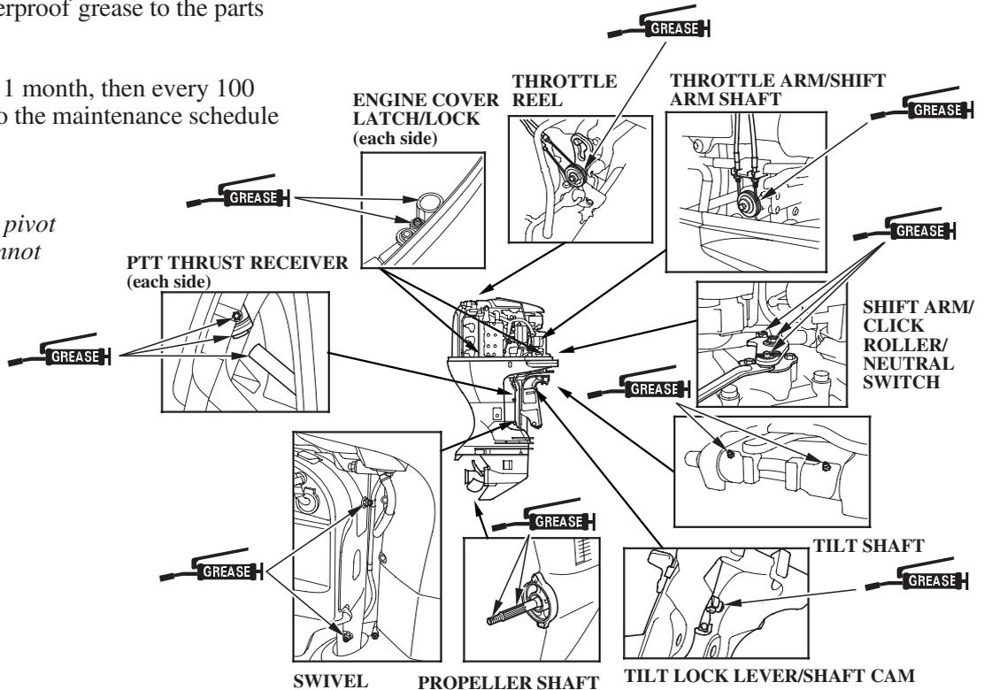
Apply corrosion inhibitor to all areas under the engine cover and any exposed metal surfaces except the belts.
