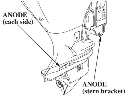
The anodes are made of a sacrificial material that helps to protect the outboard motor from corrosion.
