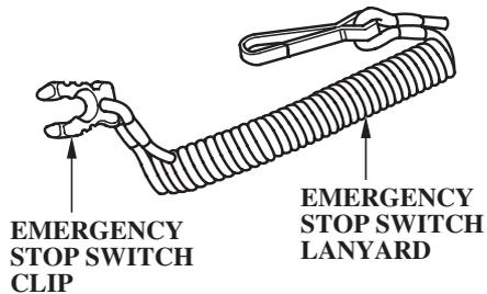
The emergency stop switch clip must be inserted in the emergency stop switch in order for the engine to start and run. The emergency stop switch lanyard must be attached securely to the operator or to the operator's PFD (Personal Flotation Device).
