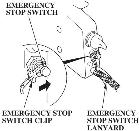
1. Put the emergency stop switch clip in the emergency stop switch, and attach the emergency stop switch lanyard securely to the operator or to the operator's PFD (Personal
