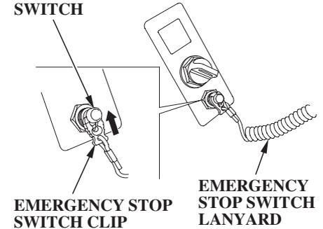
1. Put the emergency stop switch clip in the emergency stop switch, and attach the emergency stop switch lanyard securely to the operator or to the operator's PFD (Personal Flotation Device).
