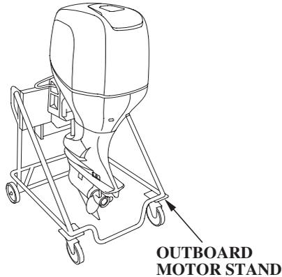
If the outboard motor will be removed from the boat for storage, we recommend storing it vertically by mounting it on a commercially available stand.
