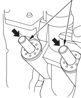
If more clearance is needed to swing the tilt lock lever into the LOCK position, rock the outboard motor forward slightly by pulling on the engine cover grip.
