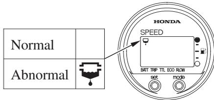
When the water separator indicator blinks:
