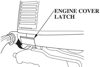
1. Unlock and remove the engine cover.
