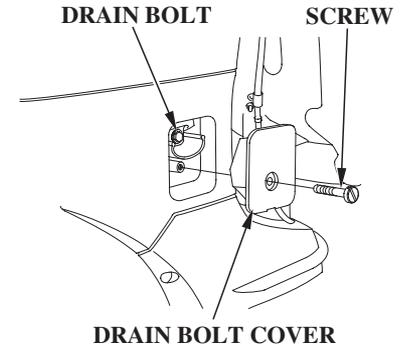
2. Remove the screw from the drain bolt cover, and remove the cover.
