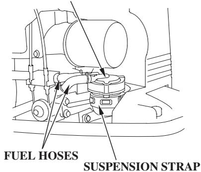
3. Remove the strainer assembly. If it is difficult to remove the strainer assembly by yourself, consult an authorized Honda Marine dealer. Remove the suspension strap from the fuel filter bracket, and then remove the strap from the fuel filter assembly.
