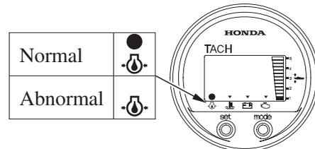
If oil pressure becomes low, the oil pressure indicator will go off, and the engine protection system limits engine speed. If you are at cruising speed, engine speed will decrease automatically.
