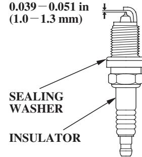
7. Inspect the spark plugs. Replace them if the electrodes are worn, or if the insulators are cracked or chipped.
