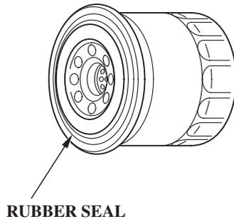
4. Clean the oil filter mounting base, and coat the rubber seal of the new oil filter with clean engine oil.
