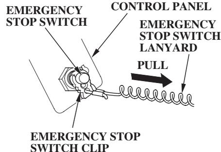
To stop the engine in an emergency, pull the emergency stop switch clip out of the emergency stop switch by pulling the emergency stop switch lanyard.
