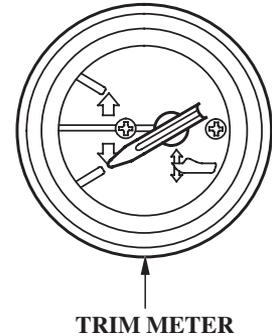
The trim meter indicates the relative trim angle of the outboard motor.
