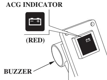
The ACG indicator turns on and the buzzer sounds in one-second intervals when the charging system is faulty.
