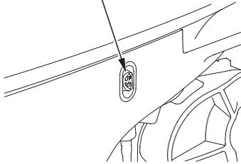
The power tilt switch is located on the engine pan. It is a rocker switch with UP and DN (down) positions for changing the angle of the outboard motor.
