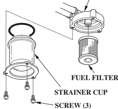
5. Remove the three screws and separate the fuel strainer cup from the strainer body.
