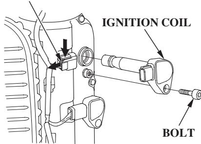
4. Disconnect the wire connector from the ignition coil by pushing on the lock tab and pulling on the connector. Pull on the plastic connector, not the wires.
