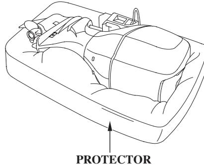
If it is necessary to store the outboard motor horizontally, drain the vapor separator (p. 85 — 86 ), and drain the engine oil (p. 65 ), before removing the outboard motor from the boat.
