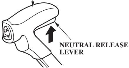
The gearshift/throttle control lever controls engine speed and selects F (forward), N (neutral), or R (reverse) gears.
