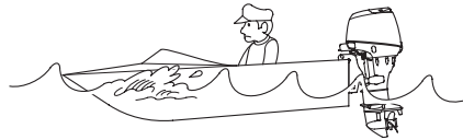
INCORRECT CAUSES BOAT TO “BOW STEER”
