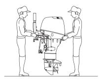
To carry, hold the outboard motor by the carrying handle, or hold by the carrying handle and the lug beneath the engine cover latch, as shown.
