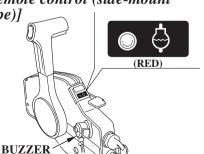
If the engine overheats, the red indicator will come on, and the engine protection system will limit engine speed. If you are at cruising speed, engine speed will decrease gradually.
