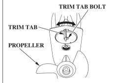
Adjust the trim tab (p. 70) with the engine stopped. Loosen the trim tab bolt above the trim tab, turn the trim tab, and then tighten the bolt securely.
