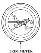
The trim meter indicates the relative trim angle of the outboard motor.
