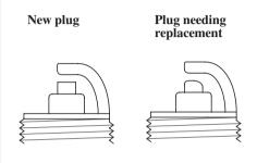
4. Inspect the spark plugs. Replace them if the electrodes are worn, or if the insulators are cracked or chipped.
