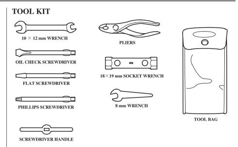
Individual items in the tool kit shown above can be purchased from an authorized Honda Marine dealer and may be used for simple maintenance procedures and/or emergency repairs. Keep this tool kit or an equivalent onboard, so that they will always be available if you need them.
