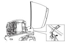
The engine cover latches fasten the engine cover to the outboard motor.
