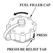
4. The fuel filler cap will lock again. Press down the pressure relief tab, and turn counterclockwise to remove the fuel filler cap.
