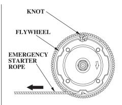
4. Set the knot at the end of the emergency starter rope in the notch in the flywheel. Wind the rope clockwise around the flywheel, as shown.
