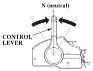
1. Move the throttle grip to the slowest speed and the gearshift lever or control lever to the N (neutral) position.
