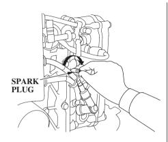
6. Install the spark plugs carefully, by hand, to avoid cross-threading.
