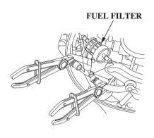
6. Remove the fuel filter from the fuel hoses.
