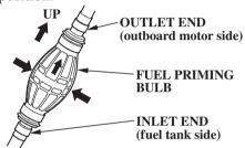
Hold the fuel priming bulb with the outlet end higher than the inlet end. Squeeze the priming bulb several times, until it feels firm, indicating that fuel has reached the carburetor.
