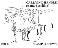
Attach the stern bracket to the boat transom by tightening the clamp screws. Push the carrying handle into the storage position. (tiller handle type)
