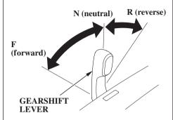
The gearshift lever is used to select F (forward), N (neutral), or R (reverse) gears.
