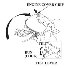
To tilt the outboard motor, move the tilt lever to the TILT position, then raise the outboard motor to the desired position by pulling on the engine cover grip.
