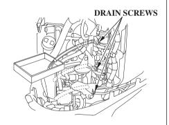
3. With the outboard motor in a vertical position, place an approved gasoline container below the fuel drain outlet, and use a funnel to avoid spilling fuel.
