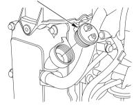
4. If the oil level is low, remove the oil filler cap, and add oil to reach the upper limit mark shown on the dipstick. Use the oil recommended on p. 74.
