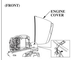
The engine cover latch fastens the engine cover to the outboard motor.
