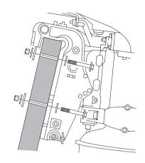
2. Secure the outboard motor with the bolts, nuts and washers.
