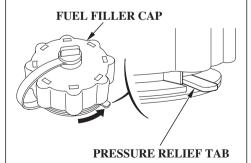
3. Press down the pressure relief tab, and then turn the fuel filler cap 1/4 counterclockwise. Release the pressure relief tab. Wait to relieve pressure.
