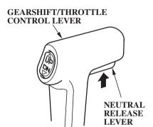
The gearshift/throttle control lever automatically locks itself in the N (neutral) position. To move the lever out of the N (neutral) position, you must squeeze the neutral release lever on the underside of the lever handle.
