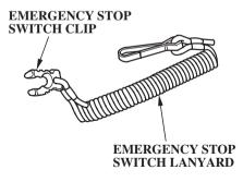
The emergency stop switch clip must be inserted in the emergency stop switch in order for the engine to start and run. The emergency stop switch lanyard must be attached securely to the operator or to the operator's PFD (Personal Flotation Device).
