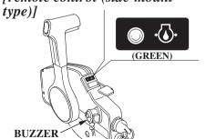
If oil pressure becomes low, the green indicator will go off, and the engine protection system will limit engine speed. If you are at cruising speed, engine speed will decrease automatically.
