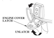
1. Unlatch the engine cover latch and remove the engine cover.
