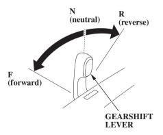
To shift gears, turn the throttle grip to the SLOW position; then move the gearshift lever to select the F (forward), N (neutral), or R (reverse) gears.
