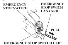
To stop the engine in an emergency, pull the emergency stop switch clip out of the emergency stop switch by pulling the emergency stop switch lanyard.
