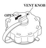
2. Turn the fuel filler cap counterclockwise so that it touches the pressure relief tab.
