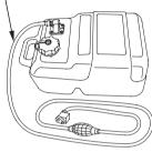
Empty the portable fuel tank into an approved gasoline container. Use a funnel to avoid spilling fuel. Rinse the fuel tank with nonflammable solvent to remove any accumulated sediment.
