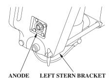
There are two anodes. One anode is located on the left stern bracket and the other anode is on the trim tab. They are made of a sacrificial material that helps to protect the outboard motor from corrosion.
