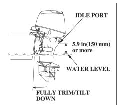
The water level must be at least 4 in (100 mm) above the antiventilation plate, otherwise the water pump may not receive sufficient cooling water, and the engine will overheat. Adverse effect to the engine can occur if the installation position of the outboard motor is too low. Trim/tilt down the outboard motor with the boat fully loaded and stop the engine. Check that the idle port is 5.9 in (150 mm) or more above the water level.
