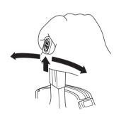
To shift gears, move the control lever to select the F (forward), N (neutral), or R (reverse) gear.
