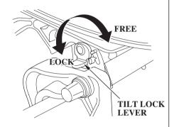
The tilt lock lever is used to support the outboard motor in the fully-raised position.
