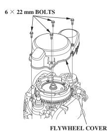
2. Remove the flywheel cover by unscrewing the four  $6 \times 22 \text{ mm}$  bolts.
