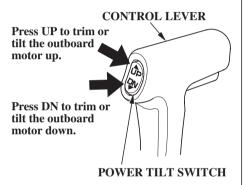
The power trim/tilt switch is located on the tiller handle or on the control lever. It is a rocker switch with UP and DN (down) positions for changing the angle of the outboard motor.
