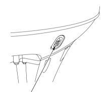
POWER TILT SWITCH (SRT and LRT types)
