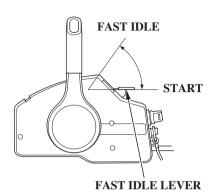
3. To start a cold engine, leave the fast idle lever in the START (fully lowered) position.
