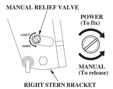
The outboard motor can also be tilted manually after opening the manual relief valve. This feature enables the outboard motor to be tilted up or down when no battery is connected. Check that nobody is under the outboard motor before opening the manual relief valve is loosened (turned counterclockwise) when the outboard motor is tilted up, the outboard motor will suddenly tilt down.
