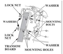
You may further secure the outboard motor by bolting the stern bracket to the boat transom. Use the mounting bolts and nut kit or other good quality stainless steel bolts, nuts, and washers. Apply silicone sealant to the bolt holes.
