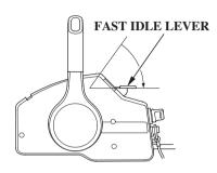
6. If the fast idle lever was used to start the engine, gradually lower the lever as the engine warms up.
