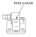
A fuel gauge is built into the fuel tank connector of the portable fuel tank.
