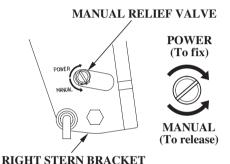
The outboard motor can be tilted manually after opening the manual relief valve. This feature enables the outboard motor to be tilted when no battery is connected.
