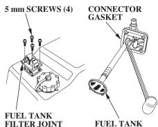
1. Remove the four 5 mm screws using a flat screwdriver, then remove the fuel hose connector and fuel tank filter from the tank.
