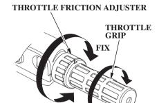
Use the throttle friction adjuster to help hold a constant throttle setting while cruising.
