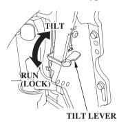
Moving the tilt lever to the TILT position allows the outboard motor to be tilted and moving the tilt lever to the RUN (LOCK) position locks the outboard motor in the desired position. Use the tilt lever to temporarily tilt the outboard motor when the boat is operating in shallow water, or mooring in shallow water. The tilt lever must be in the RUN (LOCK) position before operating the outboard motor or the outboard motor could tilt up when operating in reverse.
