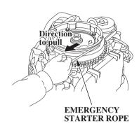
5. Pull the emergency starter rope slowly until resistance is felt, then pull briskly.
