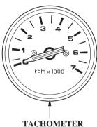
The tachometer shows engine speed in revolutions per minute.
