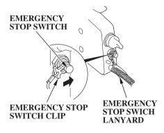
1. Put the emergency stop switch clip in the emergency stop switch, and attach the emergency stop switch lanyard securely to the operator or to the operator's PFD (Personal Flotation Device).
