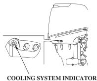
If overheating activates the engine protection system, idle the engine in neutral, and check the cooling system indicator.
