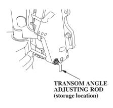
There are four transom angle adjustment positions. Three are controlled by the adjusting rod and the fourth is controlled by the stern bracket. In order to use the fourth position, remove the adjusting rod and store it in the storage location; then lower the outboard motor down to the stern bracket stop position.
