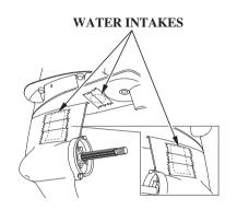
3. Cover the three water intakes with duct tape as shown above.
