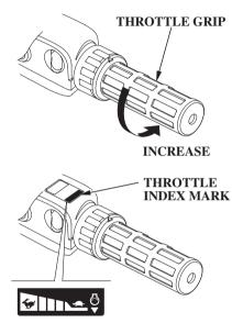
The throttle grip controls engine speed.
