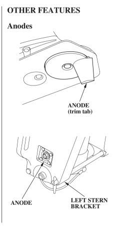
The anodes are made of a sacrificial material that helps to protect the outboard motor from corrosion.
