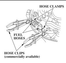
5. Place commercially available hose clips on the fuel hoses on each side of the filter to prevent fuel leakage when the fuel hoses are disconnected.
