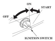
The ignition switch controls the ignition system and the starter motor.
