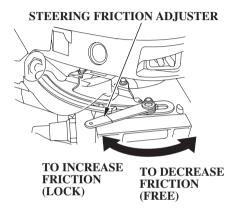
The steering friction adjuster adjusts steering resistance.
