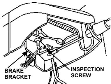
3. Release the flywheel brake lever (located on equipment), and verify that there is a strong resistance when pulling on the recoil starter. Also verify that the governor arm is moved to the idle (slow) position and there is freeplay in the cable. The cable freeplay should be 10 - 15 mm from the centerline as shown when the cable is new.
