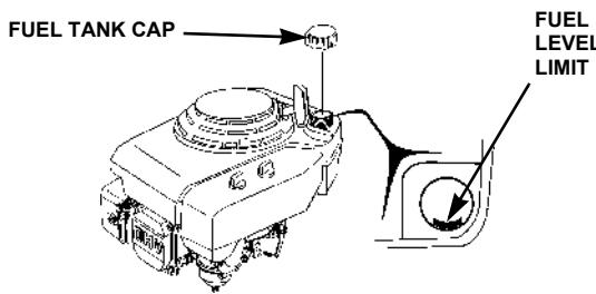
2. Add fuel to the bottom of the fuel level limit in the neck of the fuel tank. Do not overfill. Wipe up spilled fuel before starting the engine.
