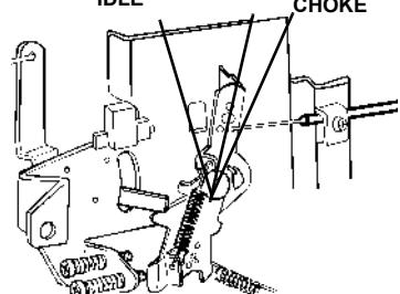
3. FOR RESTARTING A WARM ENGINE: Do not use the choke when the engine is warm.
