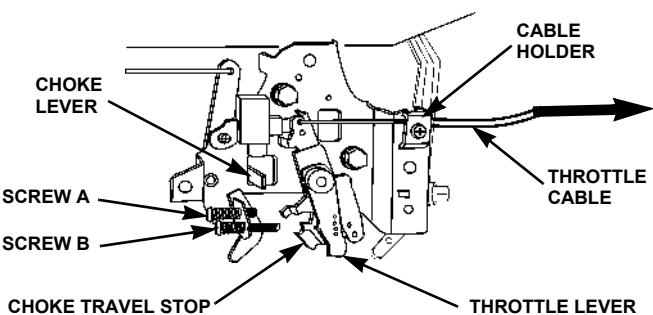
5. Move the throttle control to the choke position and verify that the engine choke rod moves the carburetor choke arm fully closed. If necessary, adjust screw B so it just contacts the choke travel stop.
