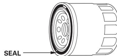
3. Clean the filter mounting base, and coat the seal of the new oil filter with clean engine oil.
