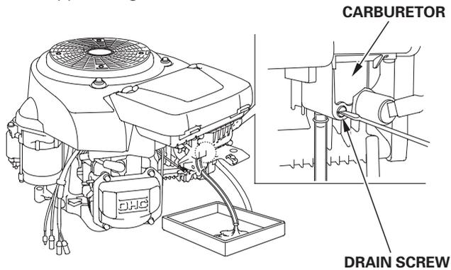
3. After all the fuel has drained into the container, tighten the drain screw securely.
