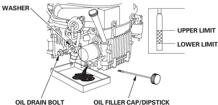
4. Install the oil filler cap/dipstick securely.
