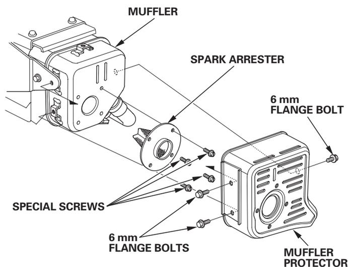
3. Use a brush to remove carbon deposits from the spark arrester screen. Be careful to avoid damaging the screen.
