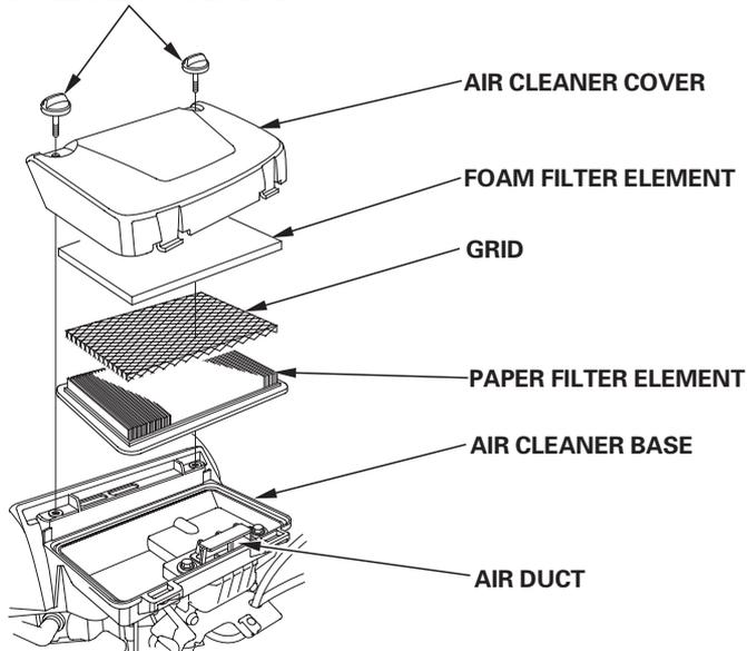
4. Inspect both air filter elements, and replace them if they are damaged. Always replace the paper air filter element at the scheduled interval (see page 6).
