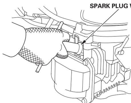
3. Inspect the spark plugs. Replace them if damaged, badly fouled, if the sealing washer is in poor condition, or if the electrode is worn.
